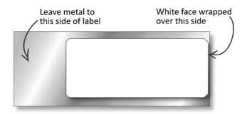
Smallest recommended bending diameter of the Confidex Silverline Blade™ is 100mm. For optimal performance please bend the label in the orientation shown below.
